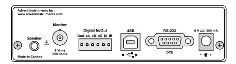
The BNC output connector can be used to monitor signals from the telephone line. Its source impedance is 600 ohms with a maximum output level of 5 Volts peak-to-peak. The 3 mm mono speaker jack to the left of the BNC monitor output performs a similar function, and can drive a speaker or headphone directly. The load impedance should be in the range of 8 to 32 ohms. Both the BNC output connector and mono audio jack have adjustable output gain and are controlled from the TRsSim software
