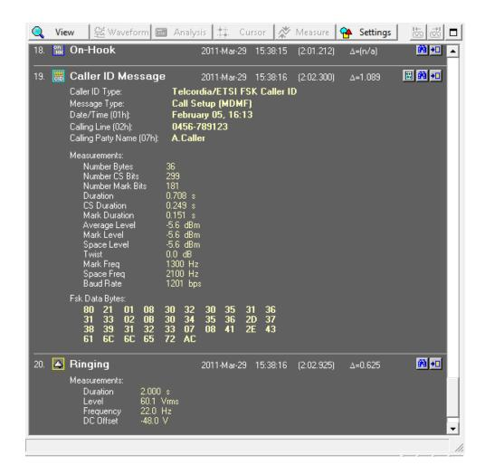
The TRsSim software includes the ability to detect and display FSK messages according to the following standards:
