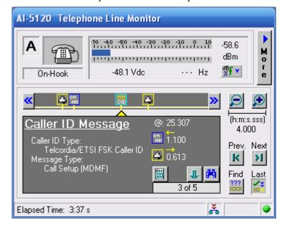
The top portion of the window displays the current line status and signal level. Both AC RMS level and DC line voltage are shown. AC signal frequency is displayed if sufficient signal level is present. Options exist to apply various signal filters (adjustable low pass, high pass, band pass, and notch) in order to minimize unwanted or interfering tones.
