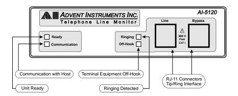
When the "Ready" indicator is illuminated (no fault condition), then the two right side LED's show when the AI-5120 has detected ringing or when the line state is in the off-hook condition. Ringing is detected if an AC voltage exceeding 40 Vrms with a frequency in the range of 10 to 100 Hz. is measured. The AI-5120 considers the line state to be off-hook if the measured voltage is below a specified threshold (by default 19 volts)
