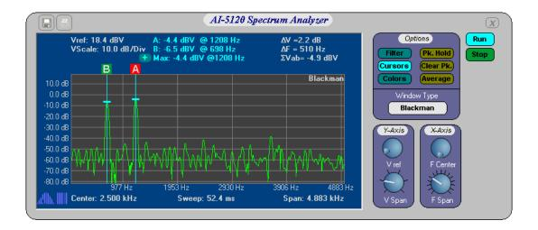
The spectrum analyzer accommodates a maximum span setting of 35 kHz. Additional features such as peak hold allow it to capture short transient like signals, while spectrum averaging assists in measuring noise levels or repetitive signals.
