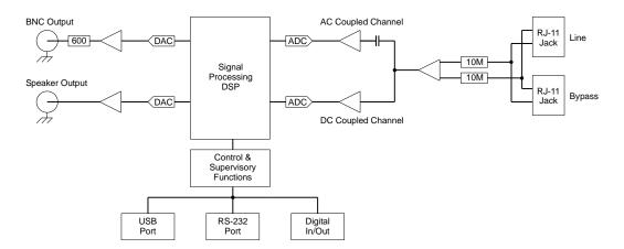
The digital samples from both AC and DC coupled channels are fed into the signal processing block. It performs all of the detection and measurement for ringing, DTMF,
