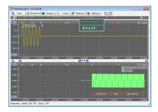
The AI-5120 records waveforms using two different channels. The first channel is DC coupled and provides a maximum range of +/- 300 volts. It is used for recording events such as ringing, on-hook, off-hook, line flash, and pulse dialing. The second channel is AC coupled with a range of 10 volts peak-to-peak. Sampling much faster than the DC coupled channel, it records the DTMF, FSK, and CAS/DTAS events.
