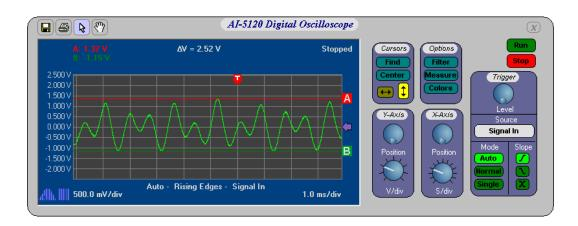
The DSO has a record depth of 5 seconds giving it the ability to capture long dialing or FSK messages, while still being able to zoom into the waveform for analyzing details.
